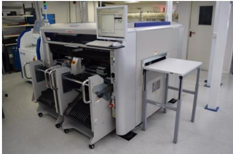
One of the new, recently installed Yamaha pick & place machines at Newbury Electronics. High res jpeg available on request.
